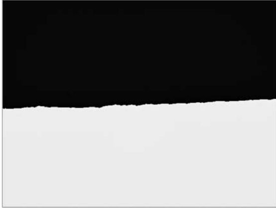
Fig. 6. Grinding wheel edge image after binarisation.
